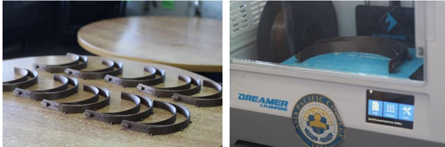
Figure 4. Face shield frames printed using 3D printer
